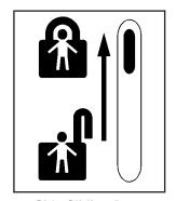
Move the button up to engage the security feature. Move the button down to return the door locks to normal operation.
